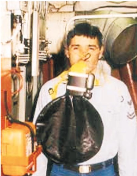
Figure 7-4. The Ocenco M20.2 shown donned and ready for escape.
