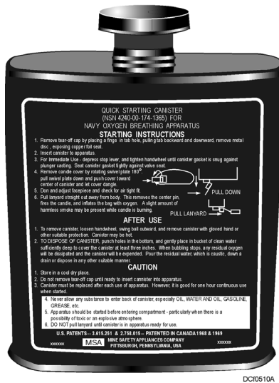
Figure 5-10. View A, front view of quick-starting canister for use with Type A-4 oxygen breathing apparatus.
