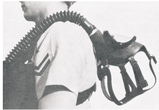
Figure 5-15. Step 4, donning the OBA.
